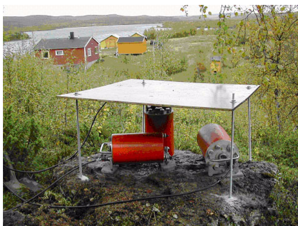
Fig. 6.4.2. This picture shows the seismometers at station Varangerbotn (VGB), before they were covered by soil, moss, and heather.
