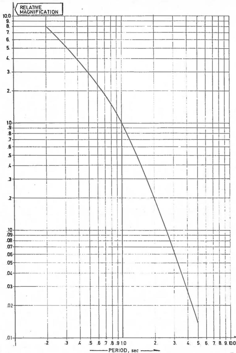
Fig. 1 Magnification of NORSAR SP Analog Station relative to Magnification at 1.0 sec period.
