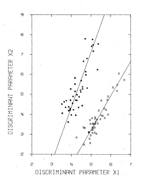
Fig. VII.8.2  $X_1:X_2$  diagram for the 46 explosions and 43 earthquakes.
