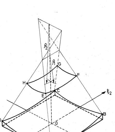
Schematic illustration of focusing effect for a perturbed wavefront. The energy flux through the areas ABCD and EFGH is the same. The principal radii of curvature of the wavefront in the latter area are  $\rho_1$  and  $\rho_2$ . The rays in the vicinity of each point of the wavefront converge or diverge to or from the two centers of curvature as shown in the figure.
