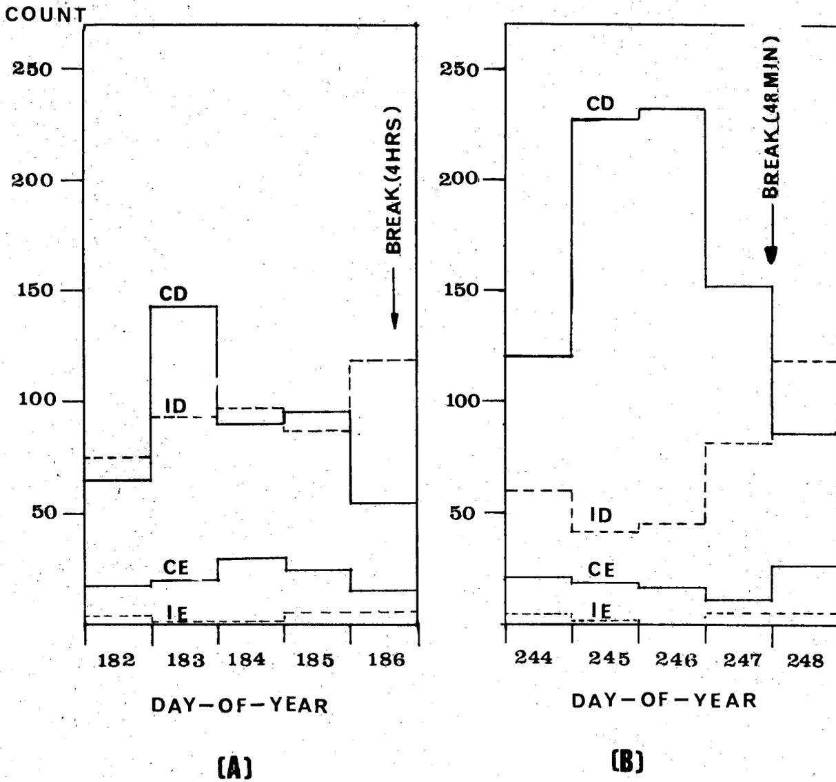
Fig. II.1.2 Variability in the coherent and incoherent detection and event rates. (A) 5 days in July; (B) 5 days in September.
