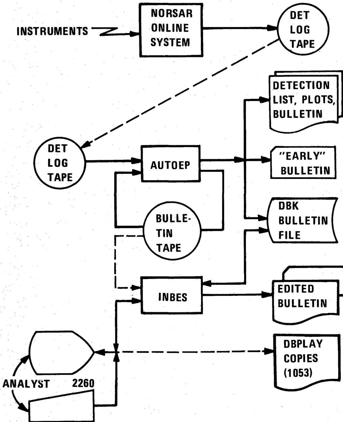
Fig. III.2.1 Data flow in the AUTOEP-INBES system
