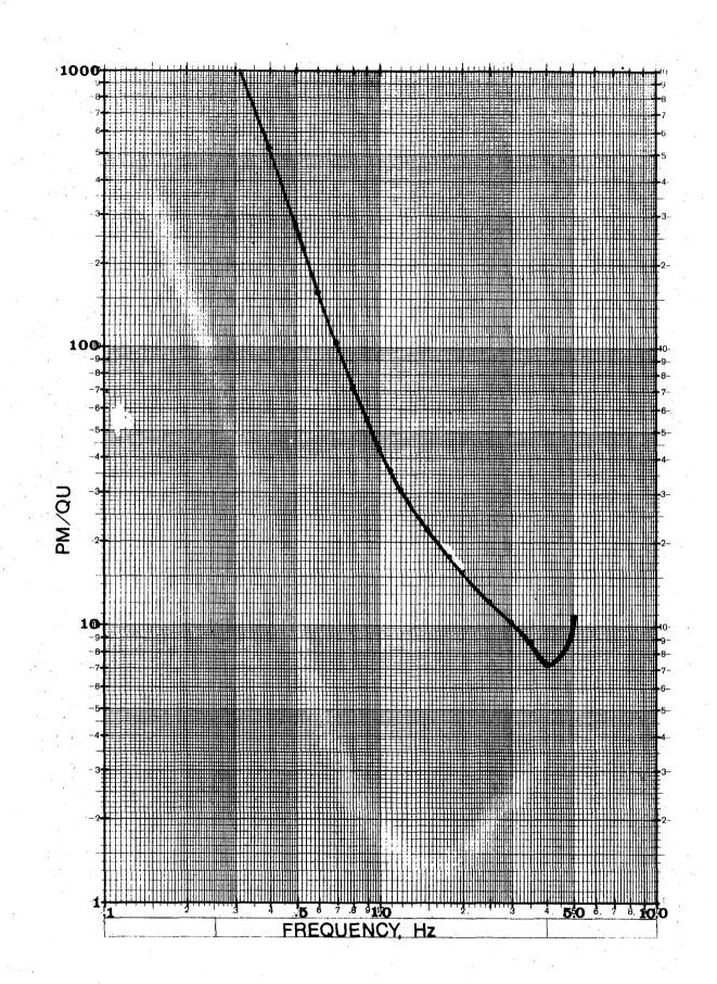
Fig. III.3.2 S-13 V frequency response.
