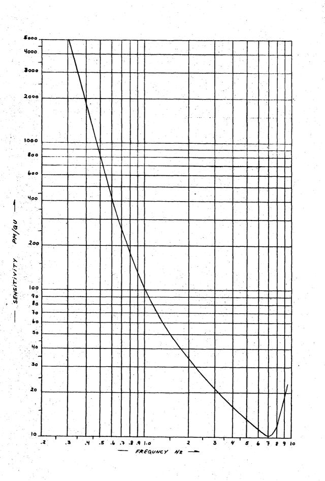
Fig. III.3.1 S-500 frequency response.
