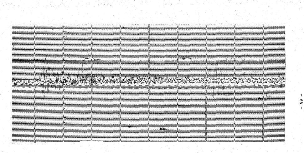
Fig. VI.8.3 Analog recording from Station 2 of the Stiegler's Gorge Seismic Network showing the disastrous Iran earthquake on 16 Sep 1978. Note especially the strong surface waves.
