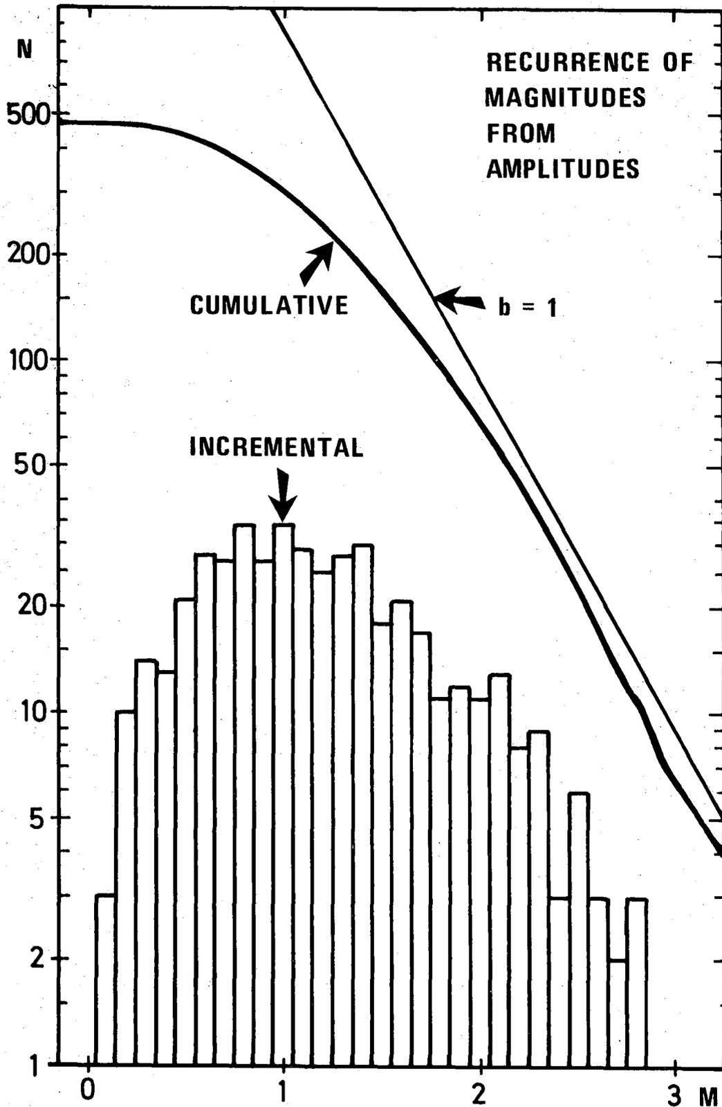
Fig. VI.9.3 Frequency-magnitude distribution for the located earthquakes in and around Svalbard, Dec 77 - May 78. The formula used is  $M = \log(A) - \alpha_1 + \alpha_2 \log \Delta + C$  where A is maximum amplitude,  $\Delta$  is epicentral distance,  $\alpha_1$  and  $\alpha_2$  are parameters, and C is a constant.
