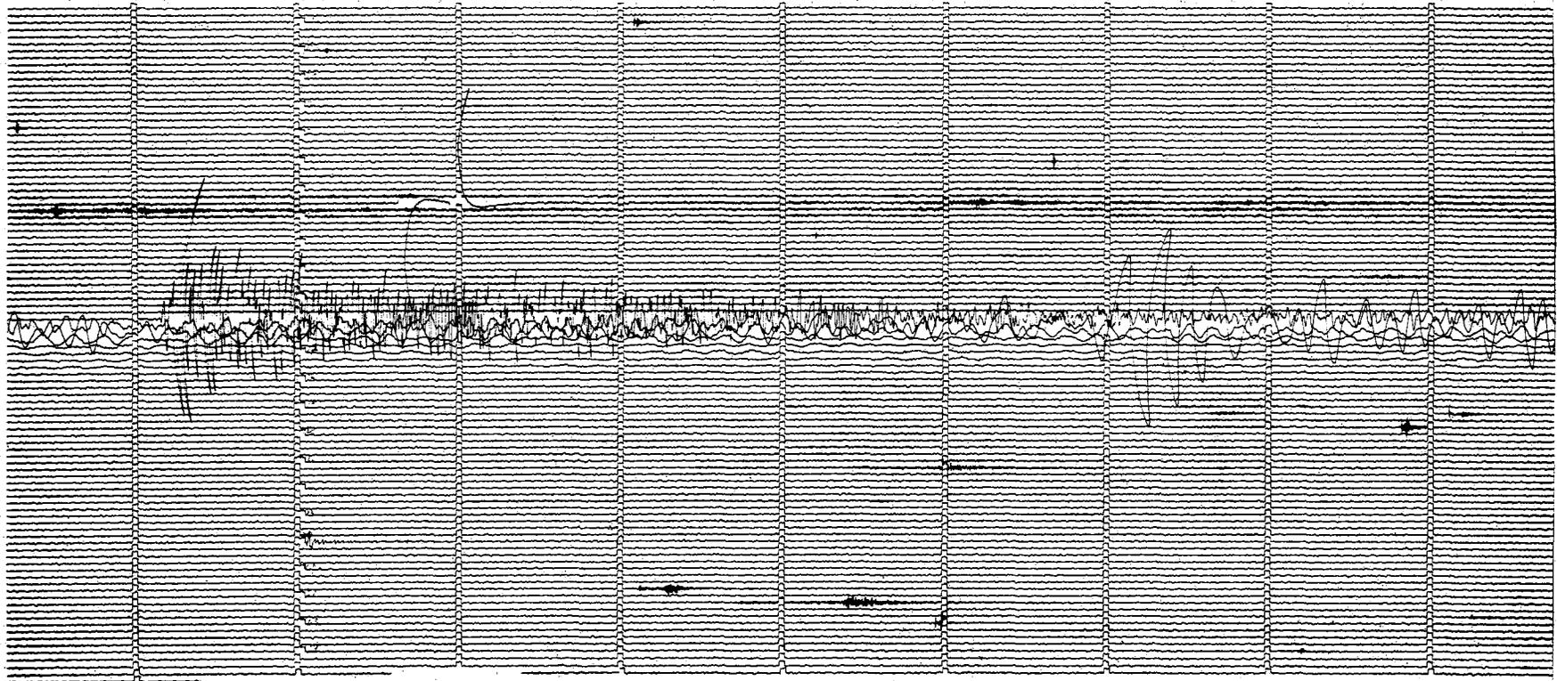
Fig. VI.8.3 Analog recording from Station 2 of the Stiegler's Gorge Seismic Network showing the disastrous Iran earthquake on 16 Sep 1978. Note especially the strong surface waves.
