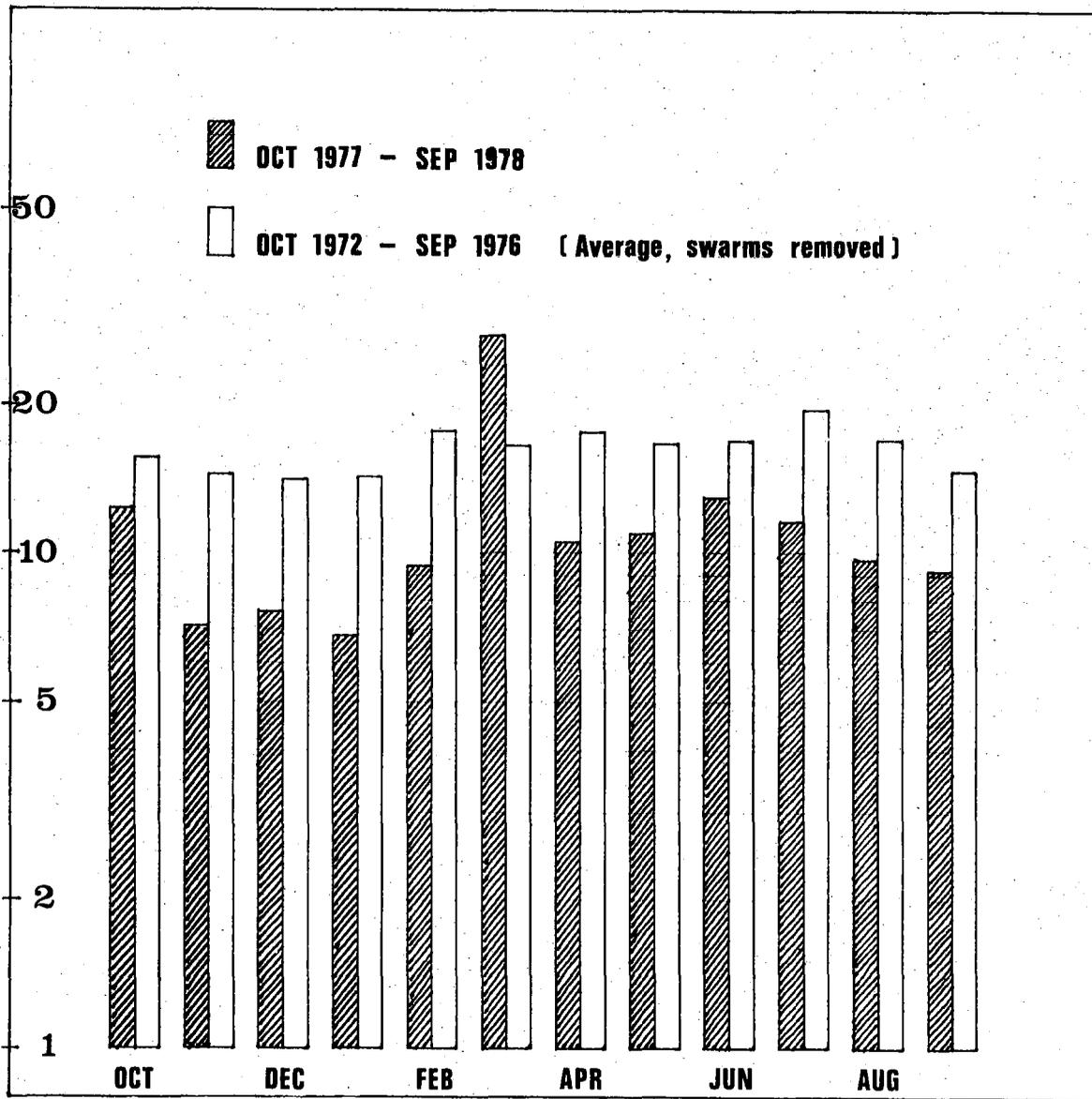
Fig. V.1.1 Monthly averages of reported events at NORSAR, corresponding to the last column of Table VI.1.1. Note that in computing the averages for the period Oct 1972 - Sep 1976 all months with significant earthquake swarms have been ignored. According to the same criterion, the month of March 1978 should be ignored when comparing the two periods.
