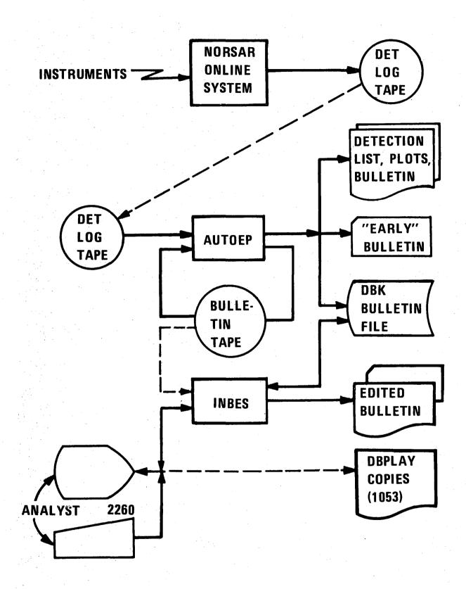
Fig. III.2.1 Data flow in the AUTOEP-INBES system
