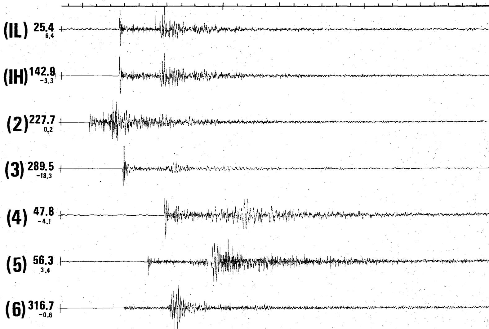
Fig. VI.8.2 A local earthquake on 17 September 1978 recorded by the Stiegler's Gorge Seismic Network. The time marks on the top are one second apart, and the first trace is a low-gain version of Station 1. The earthquake is located near Station 2 at  $7^{\circ}46.36'S$ ,  $37^{\circ}52.34'E$  and at a depth of 10.1 km. Note especially the clear onsets and the changes in polarity.
