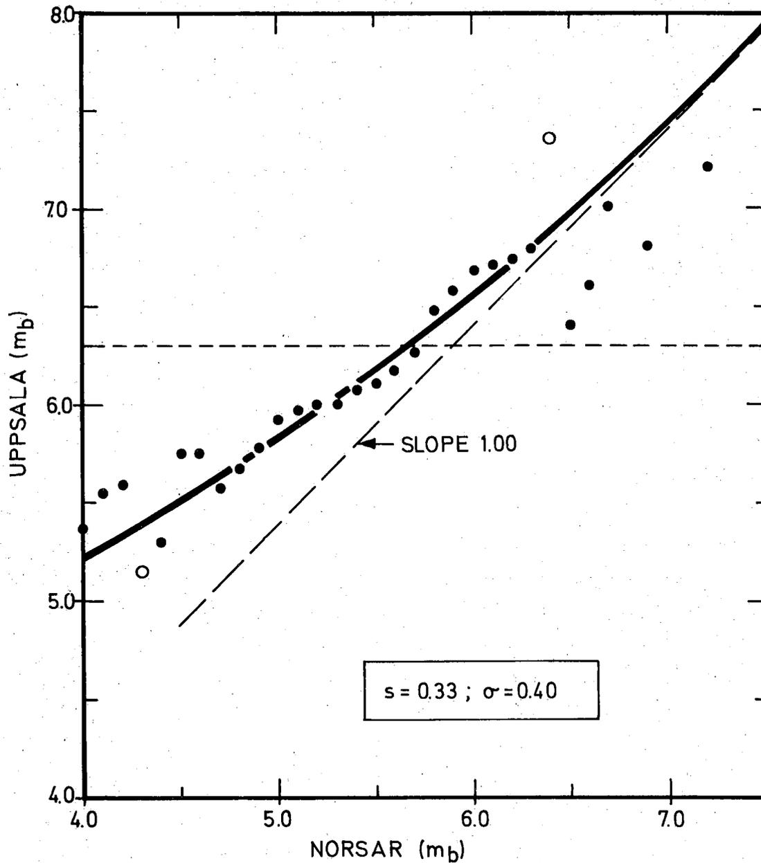
Fig. VI.3.3 Illustration of the model in Fig. VI.3.1 and VI.3.2 applied to estimate the relationship between  $m_b$  (NORSAR) and  $m_b$  (UPPSALA) (data base 386 earthquakes). The expected slope of 1.00 does not appear to fit the observed data. However, if one takes the effect of detection thresholds into account, while fixing the slope at 1.00, one arrives at the solid, curved line which is a much better fit.
