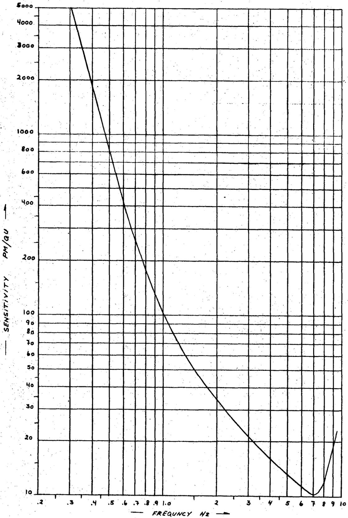
Fig. III.3.1 S-500 frequency response.
