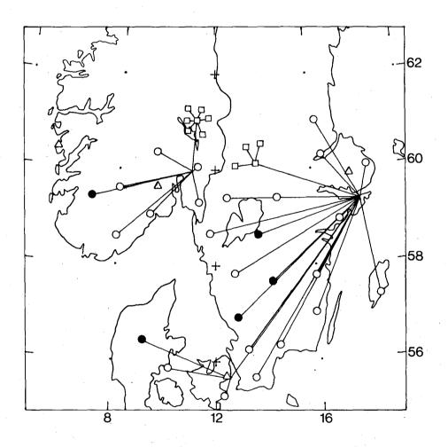
Fig. VI. 3.1 Map showing existing conventional seismic stations (triangles), array stations (squares) and planned microearthquake stations (circles, solid for three-component) in Scandinavia. The 3 microearthquake stations in Denmark and the 17 in Sweden will all have data transmitted to Stockholm, while the 7 in Norway will have data transmitted to Kjeller.
