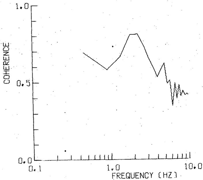
Fig. VI.4.5 Signal coherency for the data in Fig. VI.4.4. The length of the time window was 10 sec and the maximum lag in cross-correlation 15%, corresponding to about 6 degrees of freedom.
