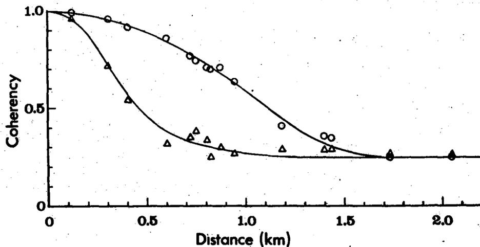
Fig. VI.4.2 Noise coherency vs distance for 1.0 Hz (circles) and 2.0 Hz (triangles). The estimates are obtained from 8.5 minutes of 20 Hz data, with 40 degrees of freedom, and an additional frequency smoothing has been applied by averaging over a frequency band of  $\pm 0.17$  octaves.
