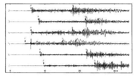
Fig. VI.3.1 Automatically determined P and S waves for three local events recorded at the Stiegler's Gorge Seismic Network. The data traces are unfiltered while the plotted envelopes are based on data filtered between 2 and 8 Hz.
