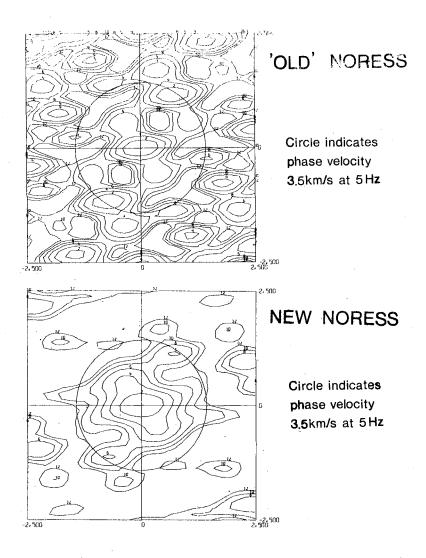
Fig. VI.1.2 Single frequency response patterns for 'old' and 'new' geometries of the NORESS array.
