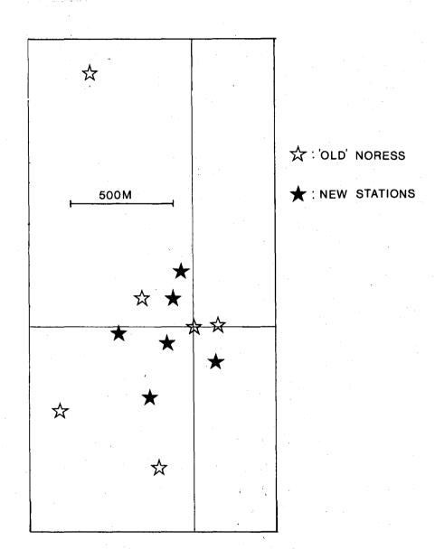
Fig. VI.1.1 Geometry of the new NORESS small-aperture array. All sensors are now equipped with 4.75 Hz low-pass filters.
