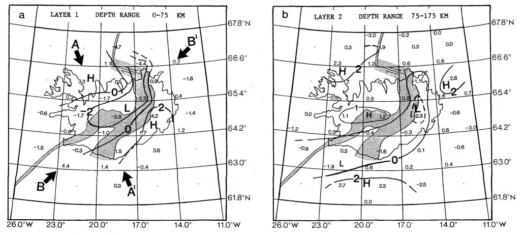
Fig. VI.3.2 (a) Velocity perturbations (in per cent) for layer 1. Areas of high and low velocities are indicated by capital letters H and L. The captial letters A-A' and B-B' together with the heavy arrows indicate vertical cross-sections through the model box as shown in Fig. VI.3.3. Resolution and standard errors for all knots are detailed in Tryggvason (1981). Figs. VI.3.1b,c & d captions as in (a) applied to the respective layers.
