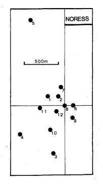
Fig. VI.3.1 Geometry of the 12-element NORESS array. All sensors are equipped with 4.75 Hz antialiasing lowpass filters.
