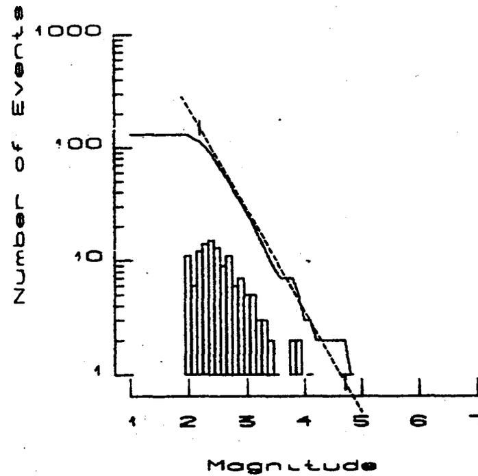
Fig. VII.4.2 Frequency-magnitude distribution for the earthquakes plotted in Fig. VII.4.1.
