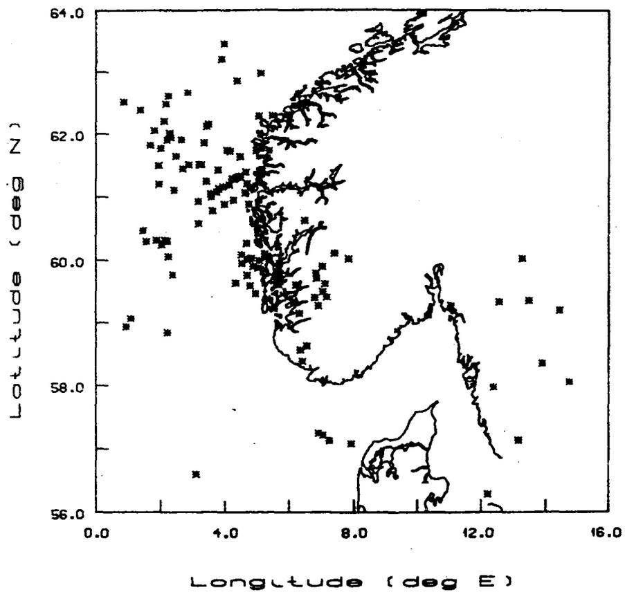
Fig. VII.4.1 Earthquake locations for earthquakes ( $M_I > 2.0$ ) reported from 1980 to 1984 using seismic stations in Scandinavia and in Great Britain.
