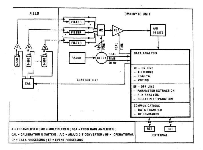
Fig. VII.6.2 The RSTE hardware configuration as detailed in text plus the essential steps involved in the data analysis centered on the powerful OMNIBYTE minicomputer. Using a multiplexer the A/D converter can handle up to 32 channels, which, if desired, permits seismometer inputs to be split in two, for example, an unfiltered and an analog-filtered channel. Such an option would reduce the CPU-load during the on-line detection processing.
