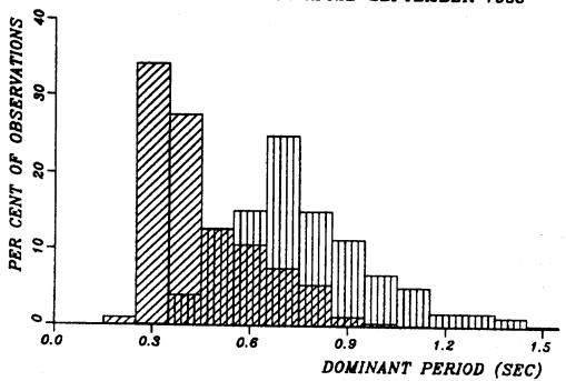
Fig. VII.4.6 Comparison of dominant signal periods estimated by NORSAR and NORESS for common events in the data base. The NORSAR histograms have vertical hatching, vs diagonal hatching for NORESS. Note the significantly lower dominant periods estimated from NORESS data.
