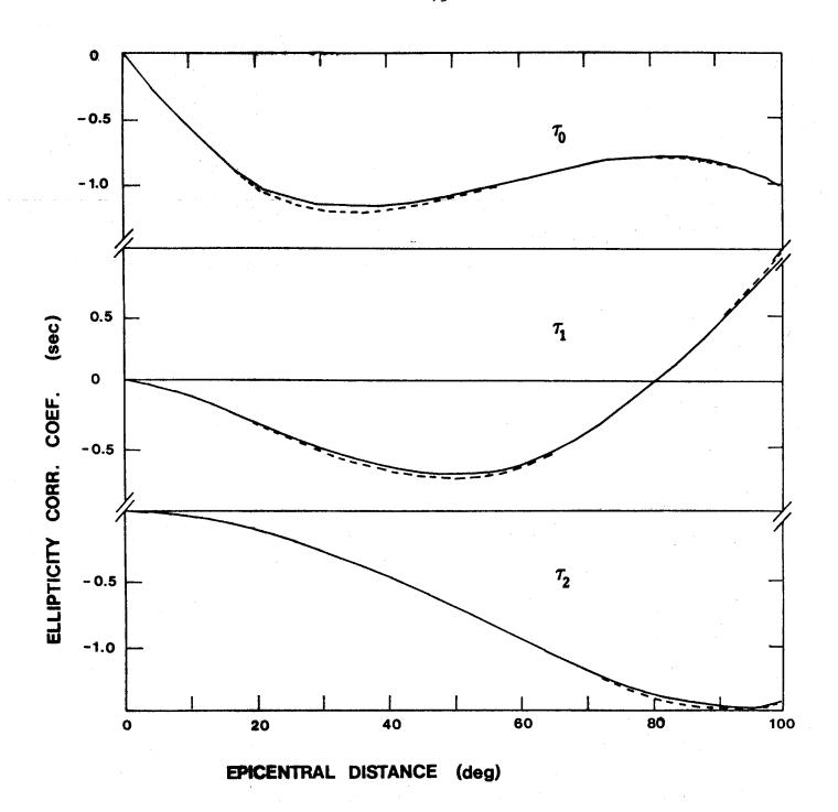
Fig. VII.6.1 Comparison of ellipticity correction coefficients for surface focus S phase
