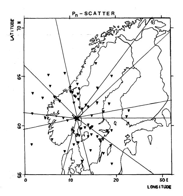
Fig. VII.10.2 Caption as for Fig. VII.10.1 except that now the wave type is Pn. Scattering sources are a bit dispersed and reflect poorer resolutin in "secondary" source locations for Pn than Pg.
