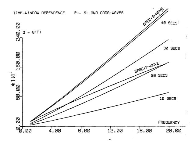
Fig. VII.7.3 Q as a function of frequency for both spectral ratio and coda-decay method. The figure shows coda Q for different time window lengths and Q for P-and S-waves using spectral ratio for a 5-second time window. Dispersion parameter u is fixed at u = 1.0, and data from both SNN- and WNN-networks are used.
