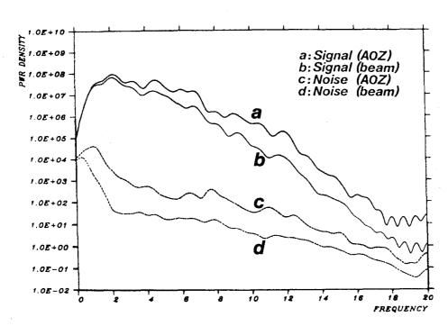
Fig. VII 5.1 The top part of the figure shows NORESS single sensor trace (instrument AOZ) and NORESS steered beam (employing the 17 seismometers AO, Cl-7, Dl-9) for Event 1 described in the text. The lower part of the figure shows power density spectra for (a) signal (AOZ), (b) signal (beam), (c) noise (AOZ) and (d) noise (beam). Tick marks on the vertical axis correspond to 10 dB power increments. The spectra have not been corrected for system response.
