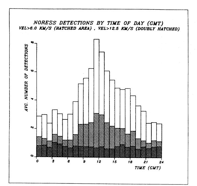
Fig. VII.3.1 Distribution of NORESS detections as a function of time of day (GMT). The average number of detections per hour is plotted, based on the time interval April-September 1985, with correction applied for system down times. The total heights of the columns correspond to all detections within the respective hours.
