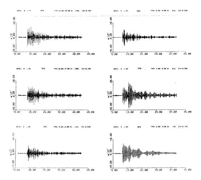
Fig VII.7.1 Examples of coda-recordings for one specific station band-pass filtered at different frequencies. The first part of the recordings indicate the noise level before P-wave arrival, and on top of the signals the RMS-envelope is drawn as an approximation to A(f,t). Axes are time after origin versus amplitude.
