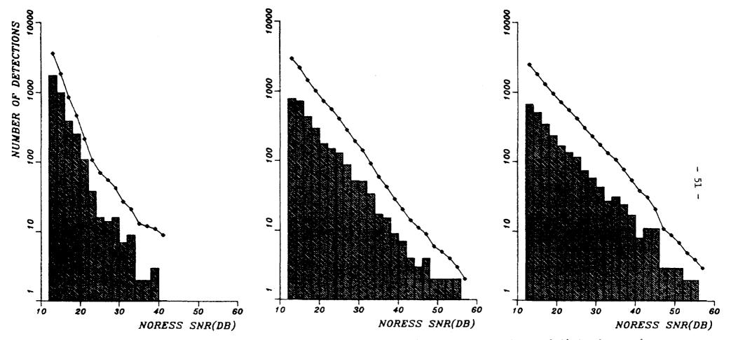
Fig. VII.3.5 NORESS detection statistics for conventional beams (nos. 1-17 of Table VII.3.1) in three velocity intervals (based on NORESS estimated phase velocity). The plots show incremental statistics (histograms) and cumulative statistics (lines). Note the differences in slopes of the logN vs SNR(DB) relations.
