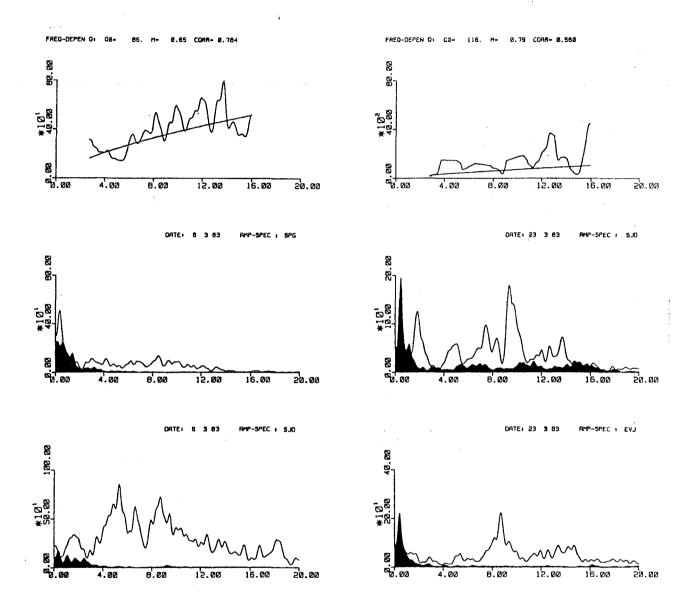
Fig. VII.7.2 Examples of spectral ratio estimation of Q for P-waves. On top the Q(f)-functions of frequency obtained from spectral ratio analysis of the two below recorded amplitude spectra. The least squares lines show the curve of the best fit frequency dependent Q. The black zones on the amplitude spectra indicate the noise before P-wave arrival.
