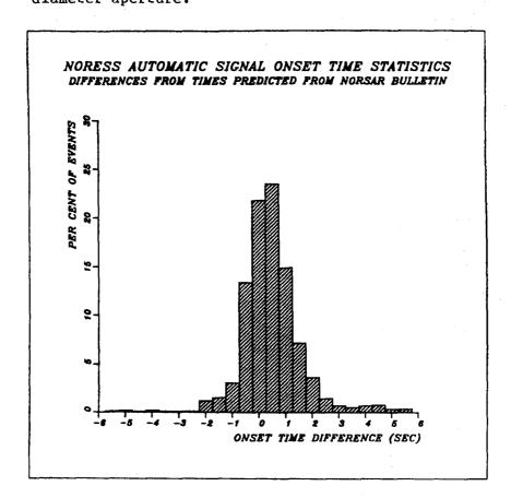
Fig. VII.4.2 Histogram showing the distribution of differences between signal onset times computed for NORESS and predicted onset times based on the NORSAR bulletin. The data base consists of seismic events detected by both systems during April-September 1985.
