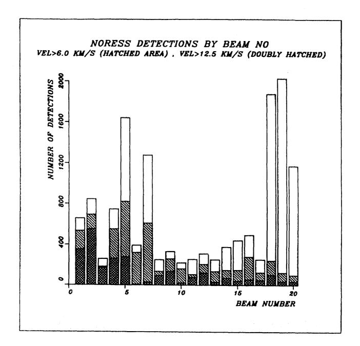
Fig. VII.3.2 NORESS detections during April-September 1985 distributed by beam number (see Table VII.3.1). For each detected phase, the beam with the largest SNR has been selected. The hatching convention is the same as in Fig. VII.3.1.
