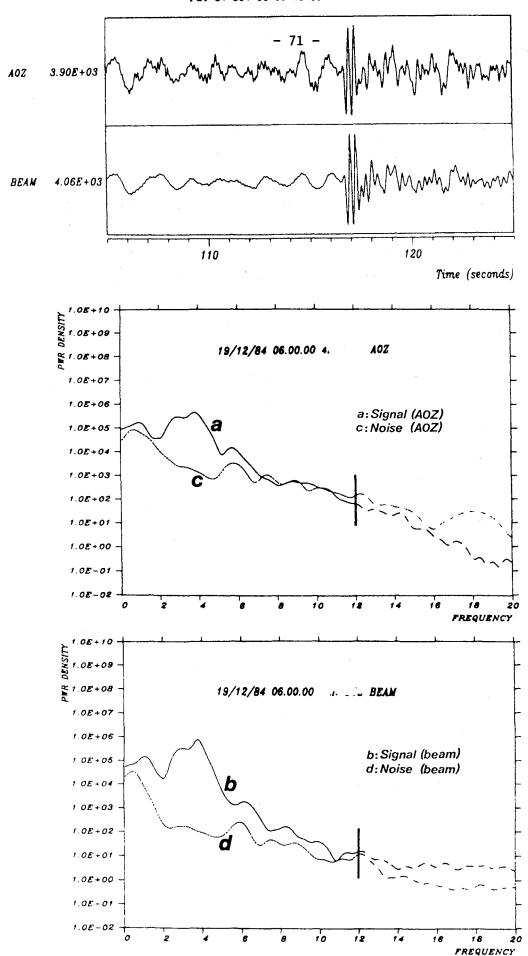
Fig. VII.5.5 Same as Fig. VII.5.1, but for Event 5 described in the text. Due to data problems, the spectra for this event are based on shorter time windows than Events 1-4, and the spectral estimates beyond 12 Hz are uncertain.
