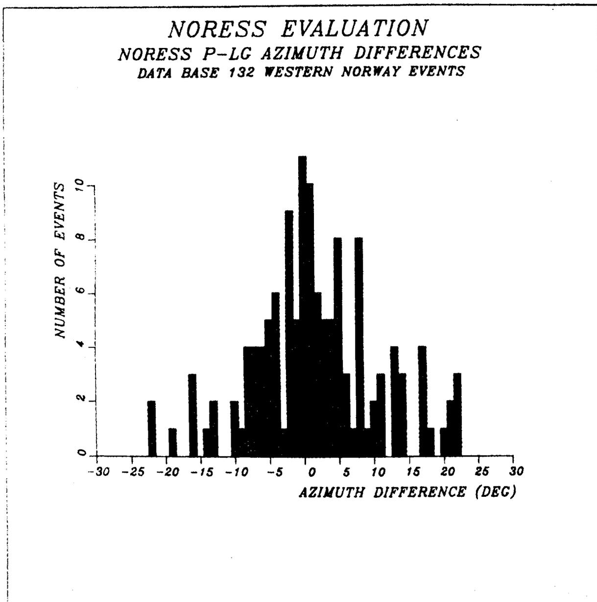
Fig. VII.2.3 The histogram shows the differences between the azimuths automatically estimated for the P and Lg phases by the routine, real time processing of NORESS data, for the 132 events in the data base.
