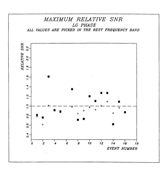
Fig. VII.3.3 Maximum SNR relative to the maximum of the AOZ, CRING and DRING configuration. The filled squares represent the beam of eight horizontal components. The crosses show the relative values of the beam with AOZ, CRING, DRING and the horizontal components, whereas the AOZ, CRING and DRING values are indicated by the dashed line at the 1.0 level.
