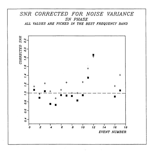
Fig. VII.3.2 Maximum corrected SNR relative to the corrected maximum of the AOZ, CRING and DRING configuration. The filled squares represent the beam of eight horizontal components. The crosses show the relative values of the beam with AOZ, CRING, DRING and the horizontal components, whereas the AOZ, CRING and DRING values are indicated by the dashed line at the 1.0 level.
