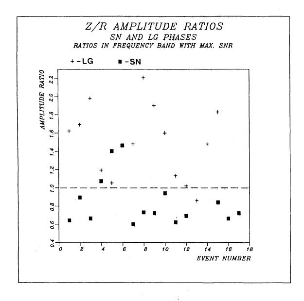
Fig. VII.3.5 Mean vertical / radial amplitude ratios for  $S_n$  and Lg phases. Only values corresponding to actually detected phases are plotted.
