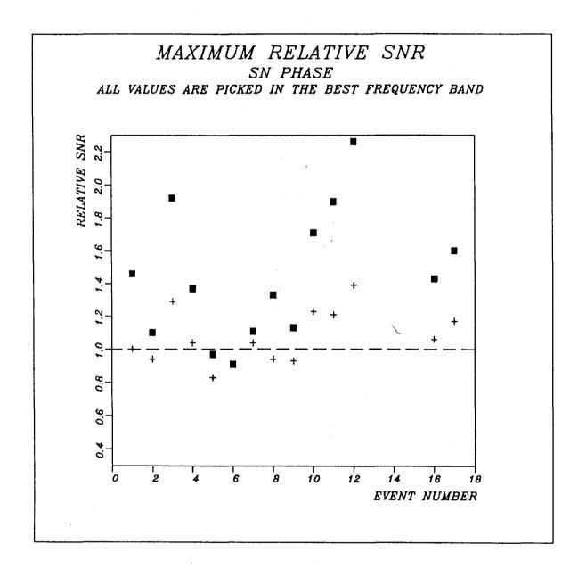
Fig. VII.3.1 Maximum SNR relative to the maximum of the AOZ, CRING and DRING configuration. The filled squares represent the beam of eight horizontal components. The crosses show the relative values of the beam with AOZ, CRING, DRING and the horizontal components, whereas the AOZ, CRING and DRING values are indicated by the dashed line at the 1.0 level.
