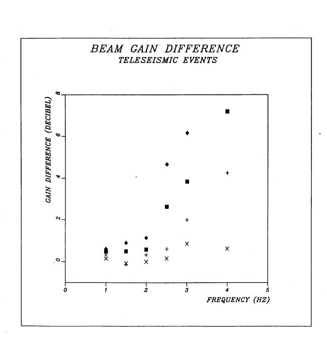
Fig. VII.4.3 The figure shows the differences between the gains for optimally steered beams and for the corresponding vertical beams. Only signals of apparent velocities above 11 km/s have been used. Symbols correspond to the ones in Fig. VII.4.2.
