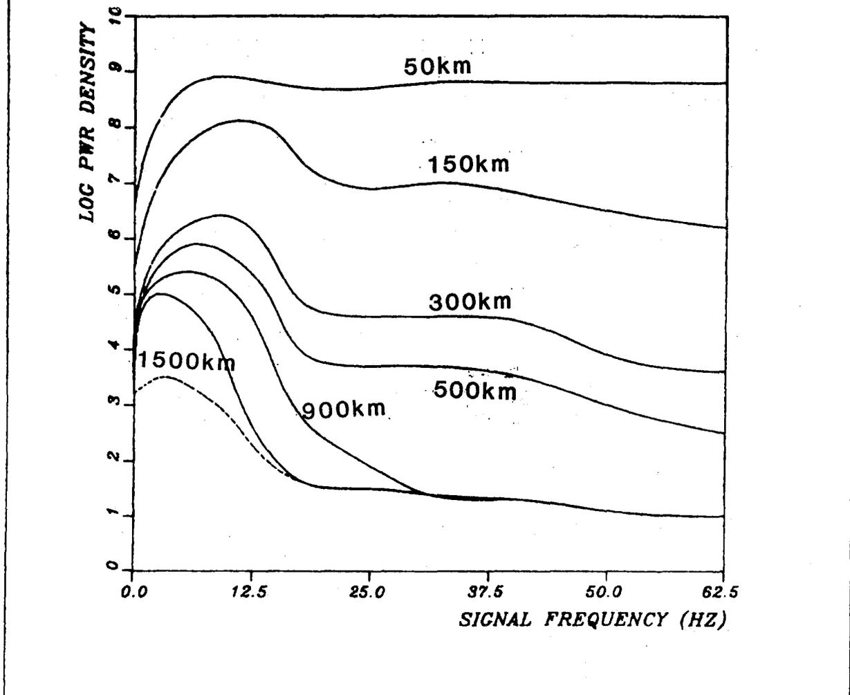
Fig. VII.2.2 Schematic illustration of high frequency P-wave spectra recorded at the HFSE, at various regional distances. The figure represents average features of about 100 regional events at various distances and azimuths, all scaled to  $M_L = 3.0$ . A typical noise spectrum is shown as a dotted line. Note that a considerable smoothing has been applied to the spectra, and that there are significant variations between individual events, even within limited epicentral areas.
