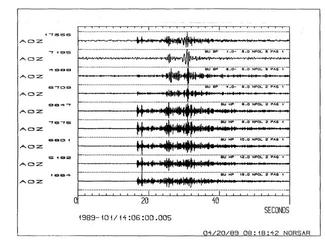
Fig. 7.5.5 NORESS single channel recording of ripple fired explosion at Sandvika (near Oslo), shown in nine filter bands. Charge was 1.615 tons over 68 delays in the time interval 0-578 ms.
