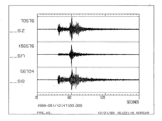
Fig. 7.5.6 ARCESS recording of ripple fired explosion at Sydvaranger, shown for a three-component station. Charge size over 200 tons.
