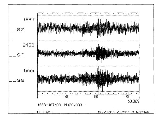
Fig. 7.5.7 ARCESS recording of ripple fired explosion at Rana Gruber. Charge was 180 tons over 34 delays in the time interval 0-1530 ms.
