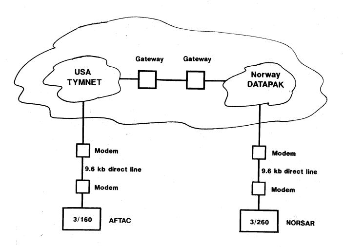
$\underline{\text{Fig. VII.6.1.}}$  Communication implemented for the new link between AFTAC and NORSAR.
