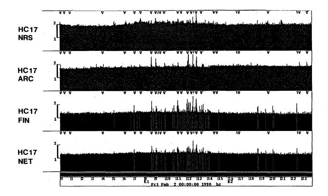
Fig. 7.6.3. The top three panels show the upper magnitude limits for mine HC17 for Friday 02/02/90, computed from the three regional arrays separately. The unit on the vertical axes is magnitude The lower panel shows the upper magnitude limit inferred from the network of arrays. The V's indicate origin times of events located by the IMS.
