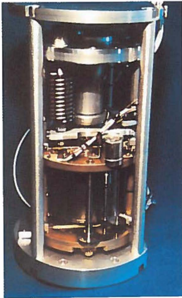
Short period seismometer designed to respond to the most detectable signals from underground explosions. The instrument is approximately 38 cm long.
