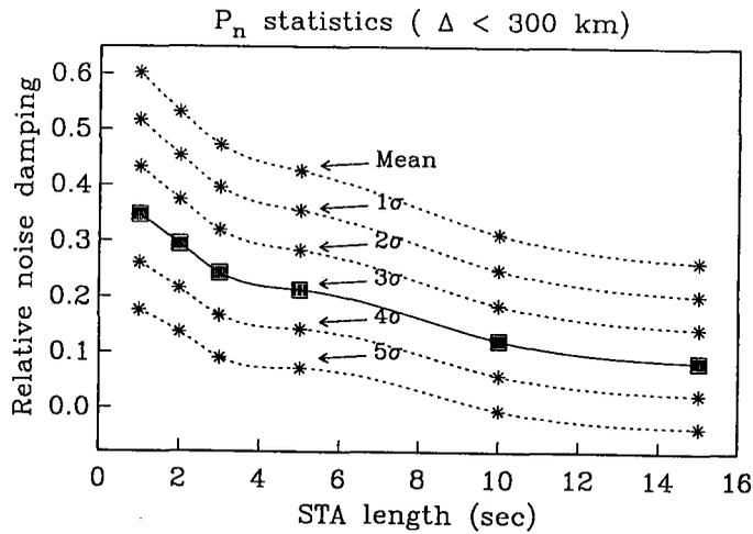
**Fig. 7.7.6.** The relative noise damping given in this figure is computed from average  $P_n$  signal behavior for events within 300 km epicentral distance (taken from Fig. 7.7.3), average noise conditions (taken from Fig. 7.7.4) and average values of noise standard deviation (taken from Fig. 7.7.5). The relative noise damping for a set of confidence levels is shown and the  $3\sigma$  level used to characterize a “worst case” situation is given by filled squares and a solid line.
