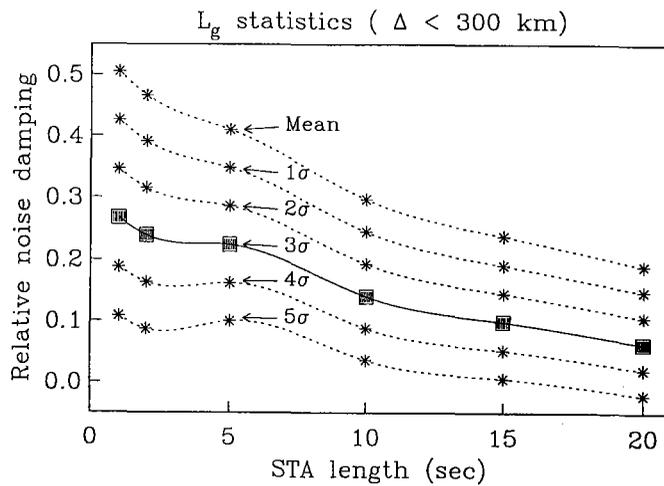
**Fig. 7.7.11.** The relative noise damping given in this figure is computed from average  $L_g$  signal behaviour for events within 300 km epicentral distance (taken from Fig. 7.7.8), average noise conditions (taken from Fig. 7.7.9) and average values of noise standard deviation (taken from Fig. 7.7.10). The relative noise damping for a set of confidence levels is shown and the  $3\sigma$  level used to characterize a “worst case” situation is given by filled squares and a solid line.
