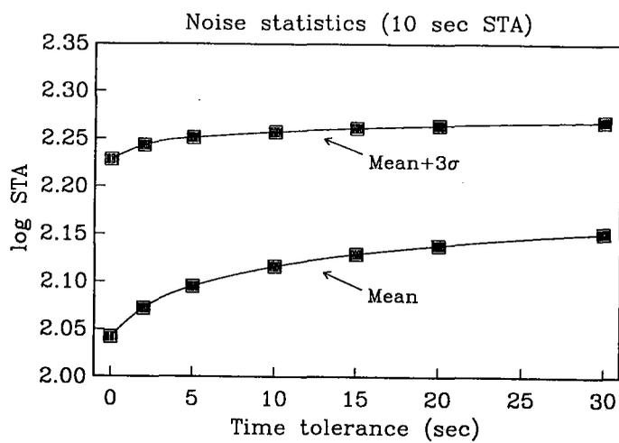
**Fig. 7.7.13.** This figure gives the mean of  $\log(STA)$  together with the mean+ $3\sigma$  level for a set of time tolerances. The first noise segment of Table 7.7.4 was bandpass filtered between 1.5 and 3.5 Hz, and the estimates were obtained using an  $STA$  length of 10 seconds.
