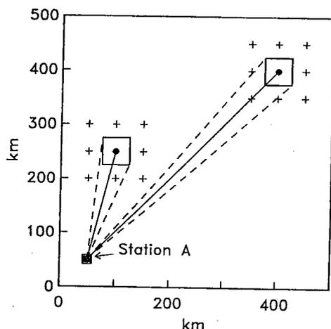
**Fig. 7.7.14.** In order to monitor a finite area surrounding each of the target points, a mis-steering in azimuth is introduced when the beams are steered towards the target points. This figure illustrates this for two target points at different distances. The azimuth deviations are indicated by dashed lines. Also note that for a fixed grid spacing, the mis-steering is a function of distance to the target points.
