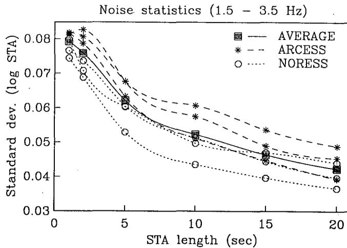
**Fig. 7.7.10.** This figure gives the standard deviation of the noise observations analyzed in Fig. 7.7.9. The average of the standard deviation curves, used for subsequent analysis of noise damping is indicated by filled squares and a solid line.
