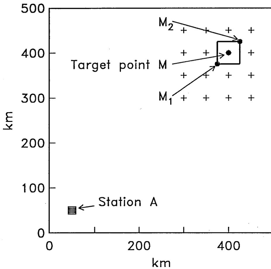
**Fig. 7.7.2.** This figure illustrates the necessity of using time tolerances. The plus signs indicate target points, and a rectangle surrounding one of the target points ( $M$ ) is also given. The point within the rectangle with the minimum travel-time is denoted  $M_1$ , whereas the point with the maximum travel-time is denoted  $M_2$ .
