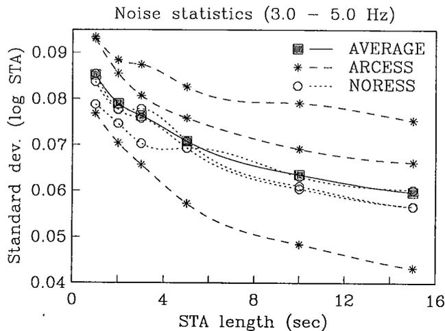
**Fig. 7.7.5.** This figure gives the standard deviation of the noise observations analyzed in Fig. 7.7.4. The average of the standard deviation curves, used for subsequent analysis of noise damping, is indicated by filled squares and a solid line.
