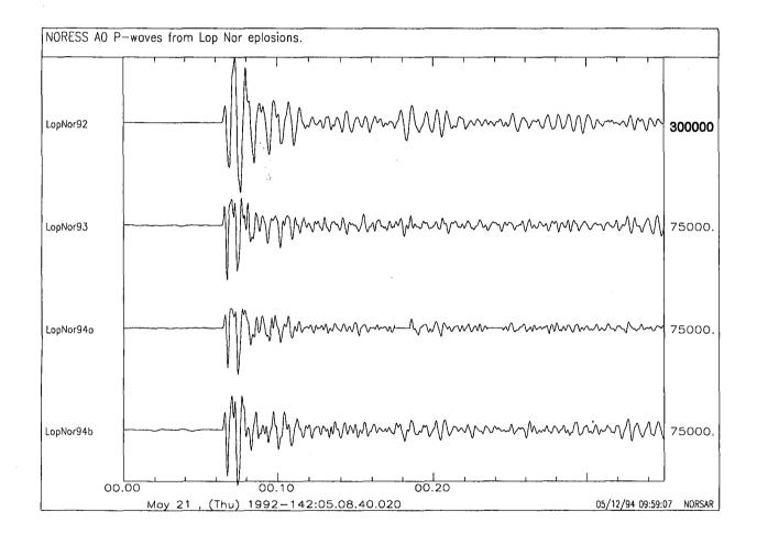
Fig. 7.2.7. NORESS P-waves (A0Z seismometer) for the four events discussed in the text. Note that the three lower traces are in the same scale, whereas the LopNor92 trace has a scaling factor that is different from the others. See Table 7.2.5 for magnitude estimates.
