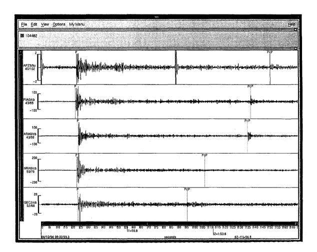
Fig. 7.2.4. P-phase waveforms of the 5 array traces (single sensor for Apatity, otherwise array beams) for the 10 June 1994 Lop Nor explosion.
