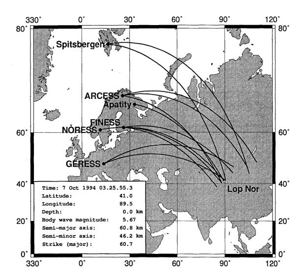
Fig. 7.2.5. Map showing the IMS solution (after analyst review) of the 7 October 1994 Lop Nor explosion. The great circle paths for the detecting arrays (based on P and PcP estimated azimuths) are also shown
