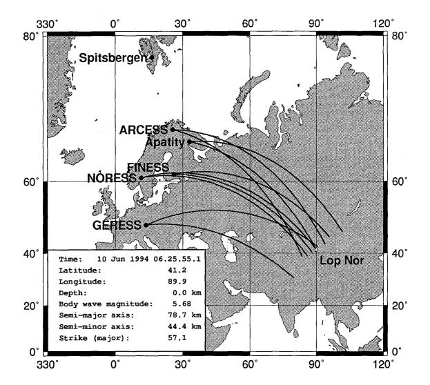
Fig. 7.2.3. Map showing the IMS solution (after analyst review) of the 10 June 1994 Lop Nor explosion. The great circle paths for the detecting arrays (based on P and PcP estimated azimuths) are also shown.
