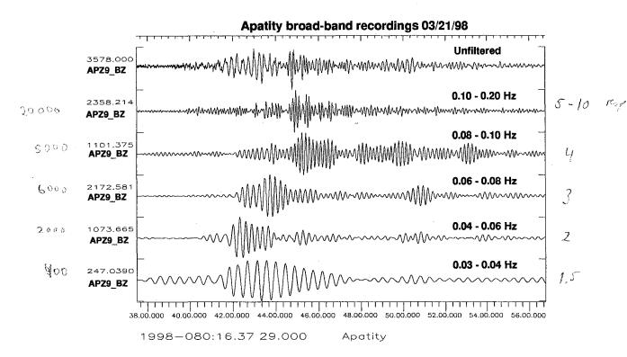
Fig. 7.4.3. Digital recording by the broad-band Guralp vertical seismometer in Apatity for an earthquake near Spitsbergen on 21 March 1998. The unfiltered data are shown in the top trace, with the other traces showing a suite of narrow-band filters applied to the recording.
