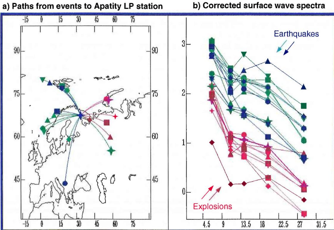
Fig. 7.4.7. Initial discrimination results using regional  $M_s:m_b$  for a data base of earthquakes and nuclear explosions with continental travel paths to the APA LP station. The left part shows the events and the travel paths to APA, whereas the right part shows surface wave spectral levels ranging from 5 to 30 second period. The spectral levels have been corrected for distance and body-wave magnitude as described in the text.
