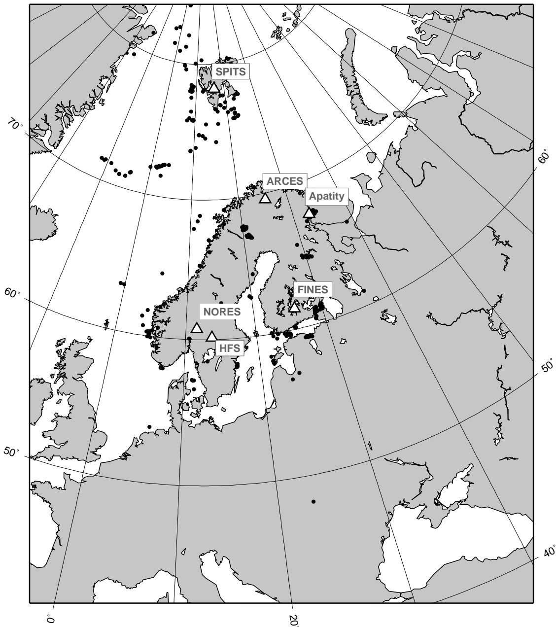
Fig. 4.2.5. The map shows the 445 events in and around Norway contributed by NOR_NDC during July - December 2006 as supplementary (Gamma) events to the IDC, as part of the Nordic supplementary data compiled by the Finnish NDC. The map also shows the main seismic stations used in the data analysis to define these events.
