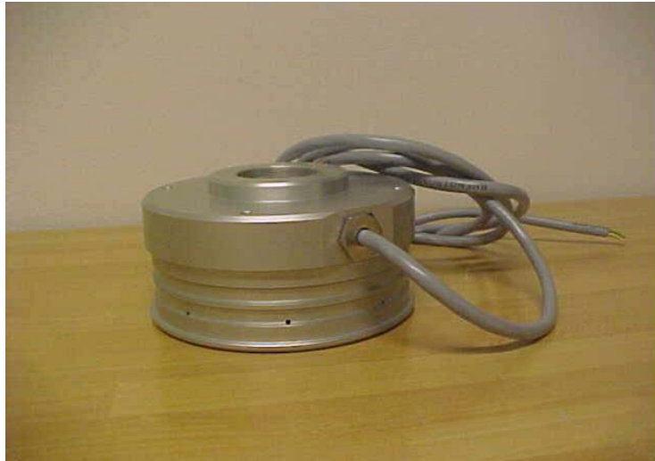
Fig. 6.4.4. The Lidstrom infrasonic microphone (After Liszka, 2007).
