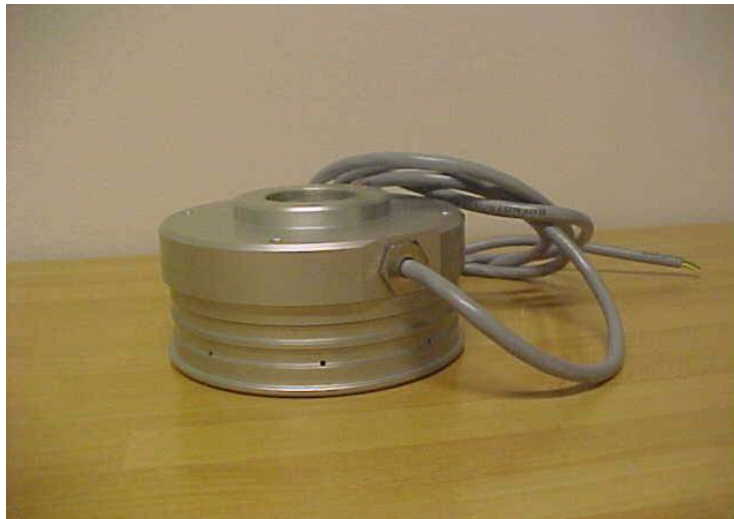
Fig. 6.4.4. The Lidstrom infrasonic microphone (After Liszka, 2007).
