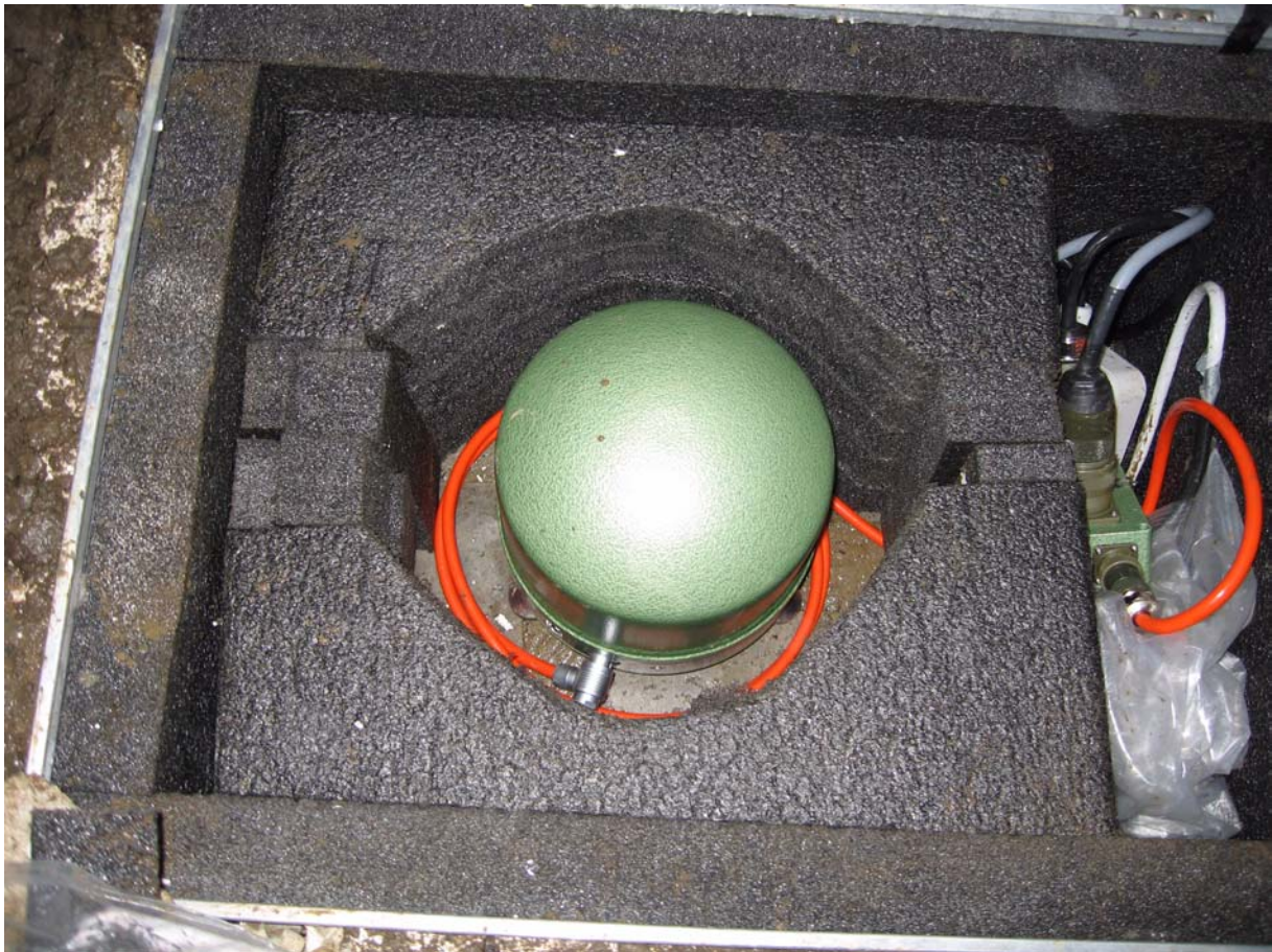
Fig. 6.3.7. The newly installed STS-2 broadband sensor at the NNSN station Hopen (Photo: Helge Johnsen, University of Bergen).
