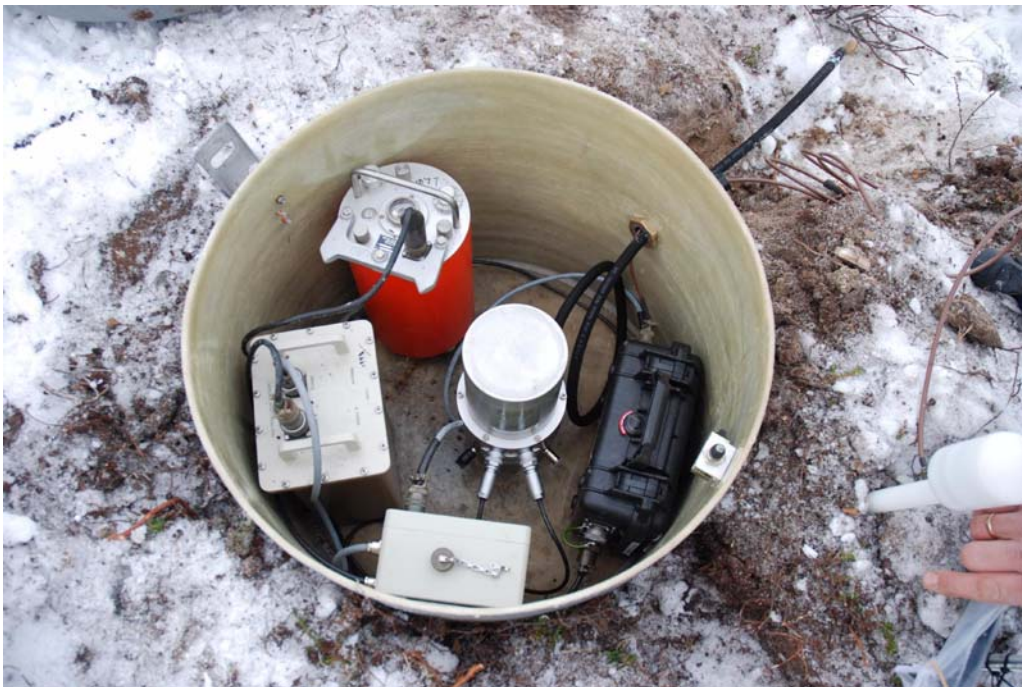
Figure 6.2.3. Pit containing a vertical seismometer with a Nanometrix digitizer and the microbarometer (middle) together with the Guralp digitizer (black box). A single inlet connects the barometer with the porous hoses arranged around the pit.
