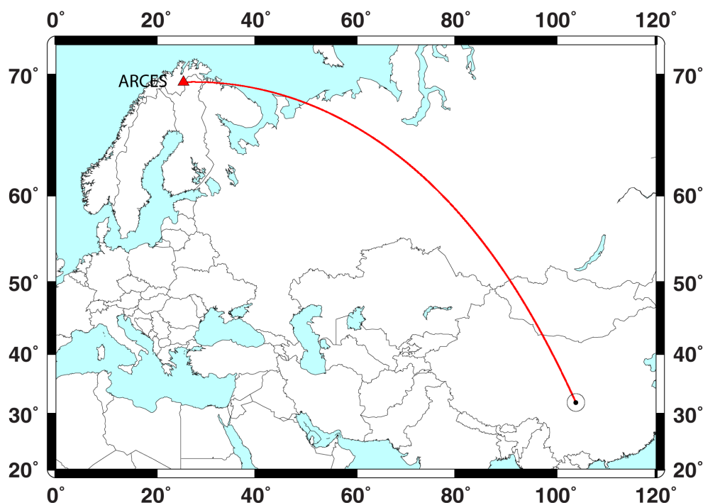
Fig. 6.3.3. The source region selected for the case study presented here is centered on 32^\circ\text{N} 104^\circ\text{E} in China, having a radius of 1.5^\circ , as shown by the open circle. The red curve shows the great circle path to the ARCES array in northern Norway, located at a distance of 56.4^\circ from the center of the source region.
