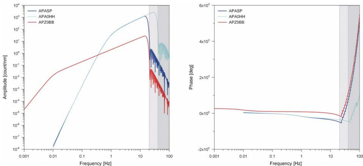
*Fig. 6.3.4. Displacement amplitude (left) and phase (right) response for the Apatity array and single 3-component station APZ9 configurations. The short-period array channels (APASP) are noted in blue, the high-frequency APA0 site channel (APA0HH) in cyan and the APZ9 broadband station (APZ9BB) in red. Shaded areas represent the range beyond the Nyquist frequency.*
