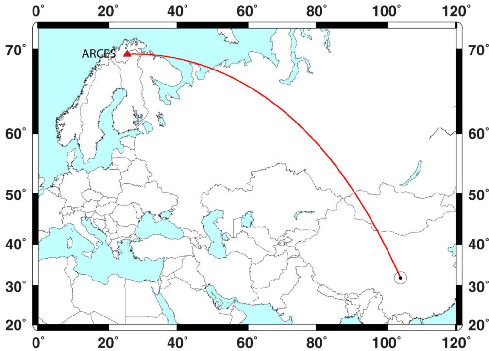
Fig. 6.1.1 The source region selected for the case study presented here is centered on 32^{\circ}\text{N } 104^{\circ}\text{E} in China, having a radius of 1.5^{\circ} , as shown by the open circle. The red curve shows the great circle path to the ARCES array in northern Norway, located at a distance of 56.4^{\circ} from the center of the source region.
