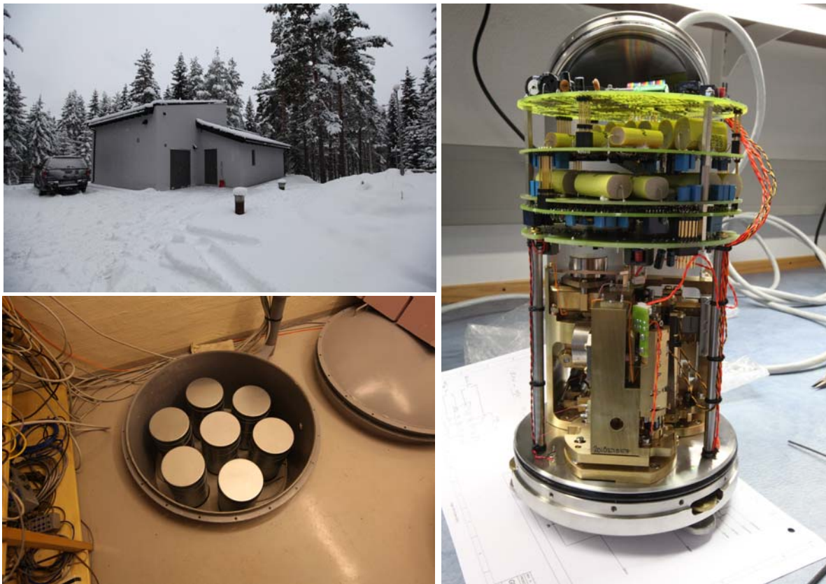
Fig. 6.4.3. Top left: Central building of the NORSAR test facility. The subsurface vault containing the broadband site NC602 and the test instruments is to the right of the building. Bottom left: One out of three pits in the vault with thermally insulated Guralp instruments. Right: An open Guralp 3T hybrid instrument.
