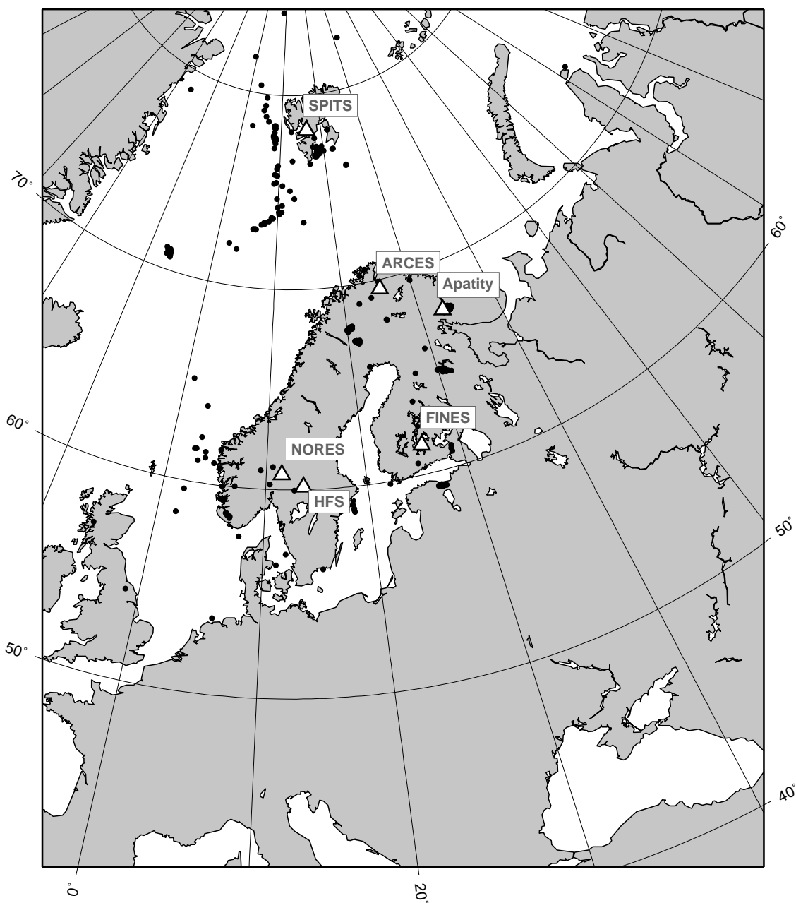
Fig. 4.2.5. The map shows the 410 events in and around Norway contributed by NOR_NDC during January - June 2011 as supplementary (Gamma) events to the IDC, as part of the Nordic supplementary data compiled by the Finnish NDC. The map also shows the main seismic stations used in the data analysis to define these events.
