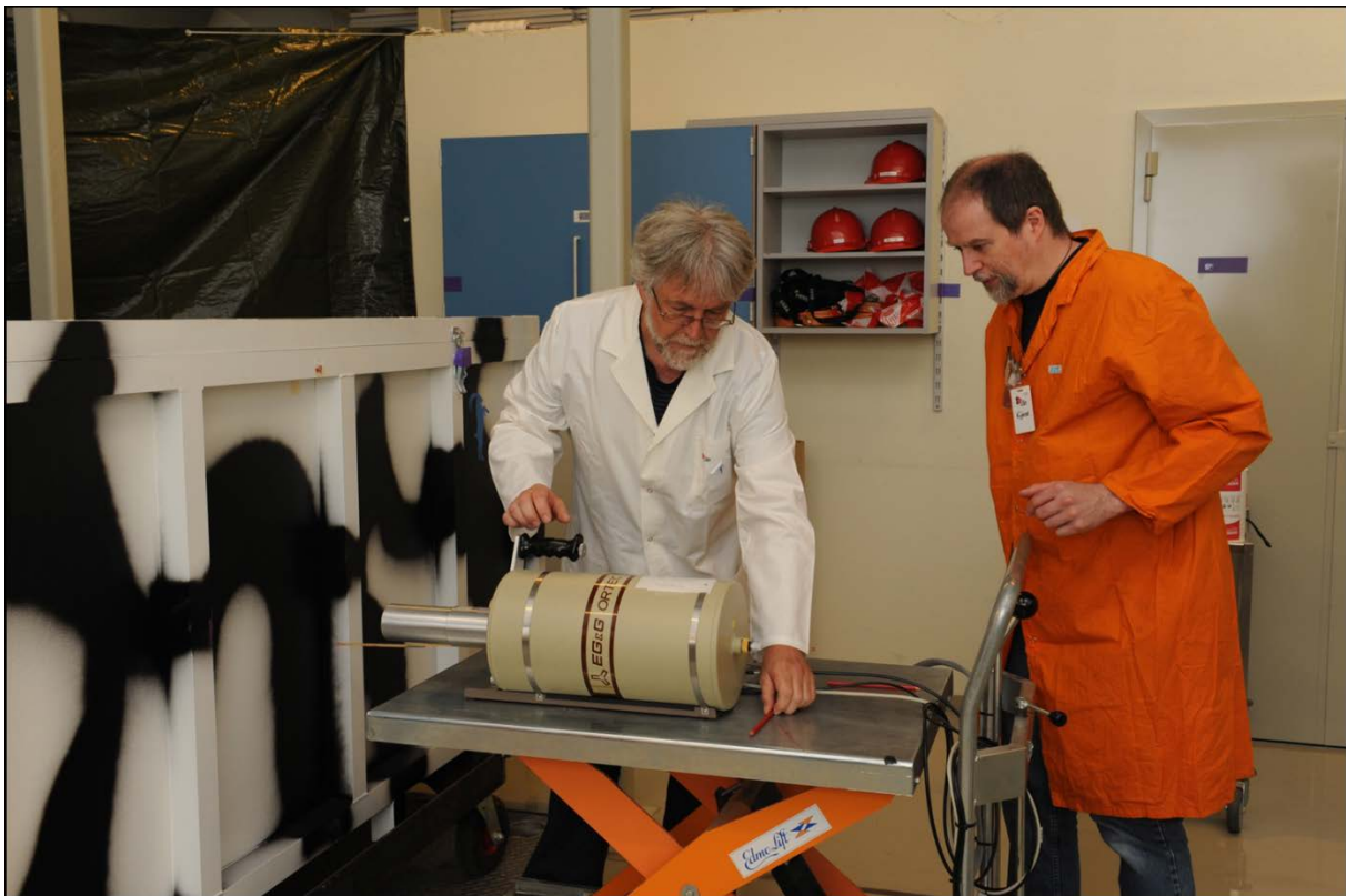
Fig. 6.4.3 An inspector watches as a host representative performs measurements using the Information Barrier system. Measurements are performed on the Odin "nuclear weapon", which is still inside the transport container.
