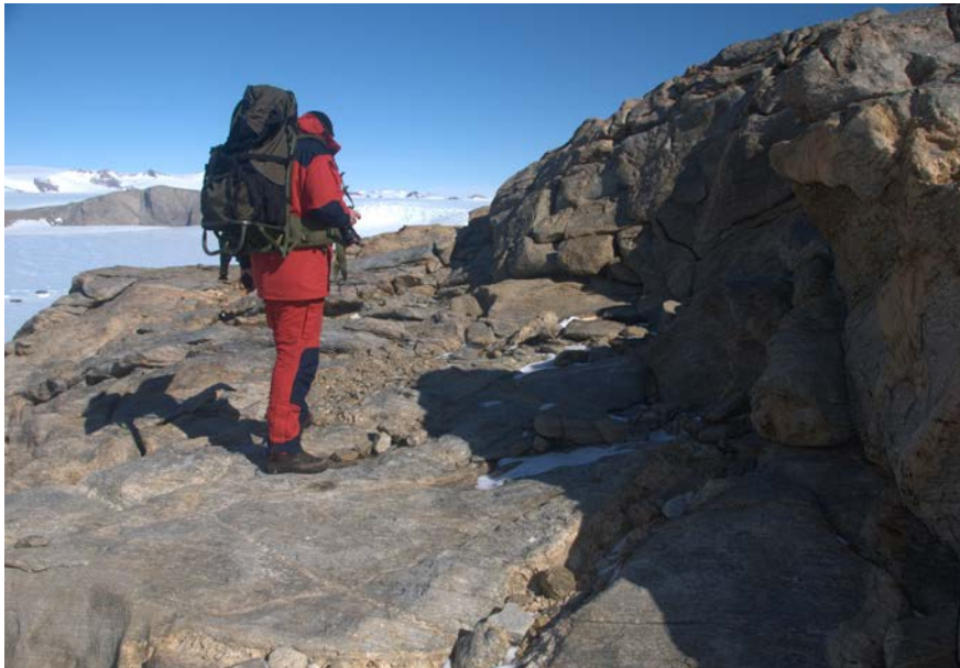
Fig. 6.2.2 The picture shows the selected seismometer site with bedrock surface and natural shielding for some directions against the strong Antarctic storms.
