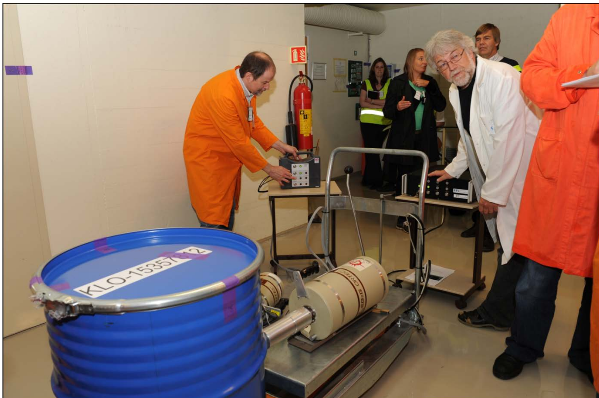
Fig. 6.4.6 Information Barrier measurements are performed on the Odin pit contained inside the blue barrel. Both Information Barrier prototypes were used.
