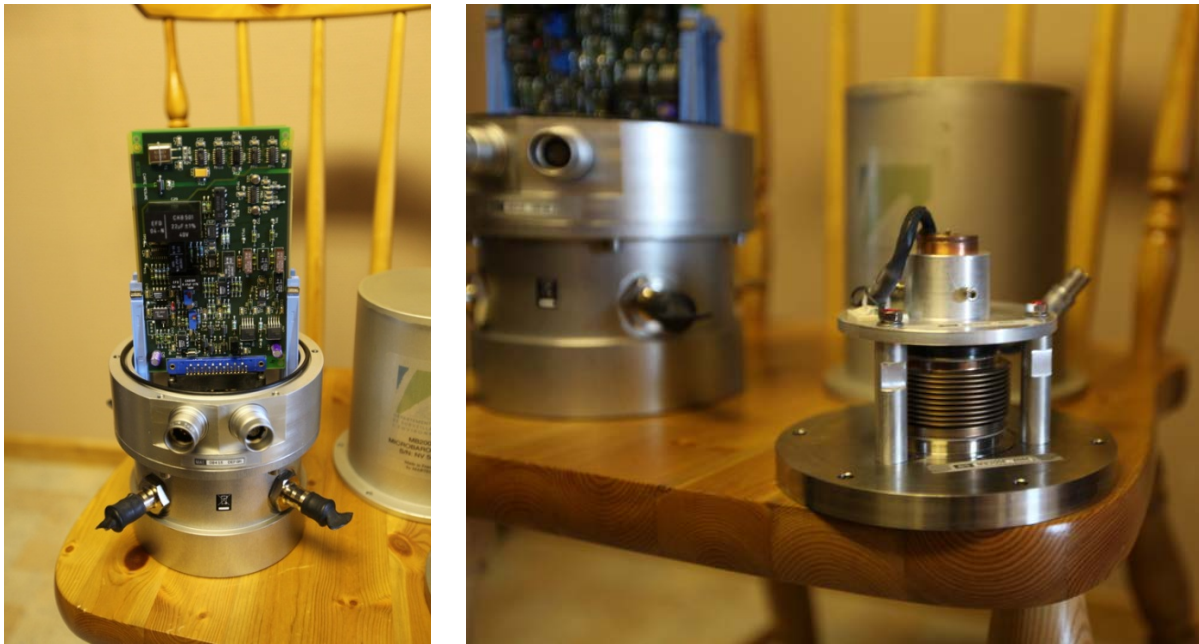
Fig. 6.4.2 Picture of an opened MB2005 sensor (left: electronic card, right: barometric aneroid bellows and displacement transducer).
