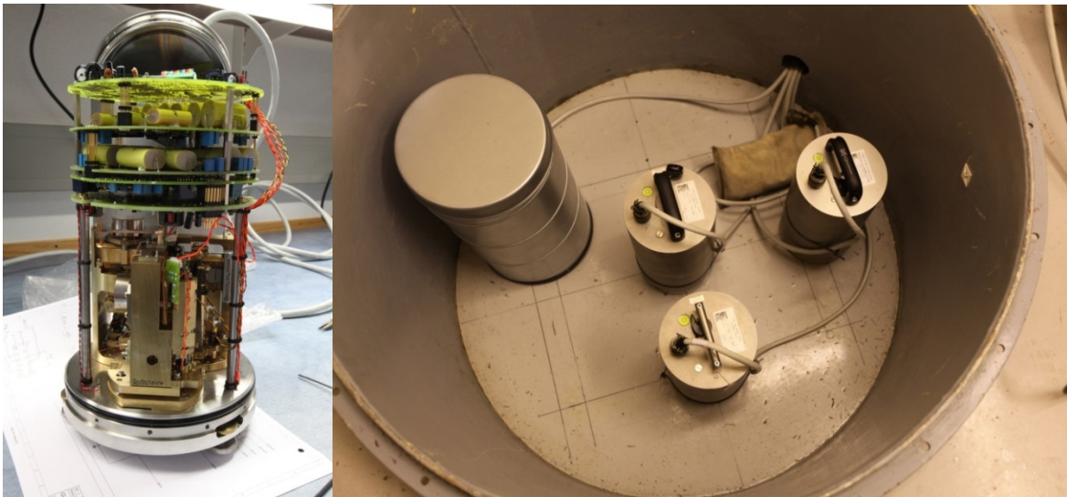
Fig. 6.2.8. Güralp CMG-3T HYBRID sensor. Left: Cover removed, right: installed in one of the vault pits. The sensor is covered with an insulation tube.
