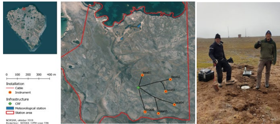
Fig. 11.7.2 To the top left is Bjørnøya, approximately 20 km in length, north to south. The six-element seismic array is located within the area shown with red borders in both maps, close to the meteorological station on the island. Right: NORSAR's Kjell Arne Løken and Jon Magnus Christensen during the array installation campaign on the island in August 2019.
