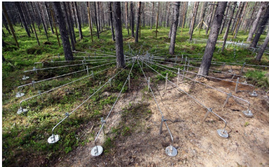
Fig. 11.2.2 Photo of one of the four steel pipe arrays at one of the ten instrument sites of IS37. As explained in the text, this design aims to reduce the effect of wind noise on the infrasound signals of interest. Note the inlet ports, looking like shower heads.
