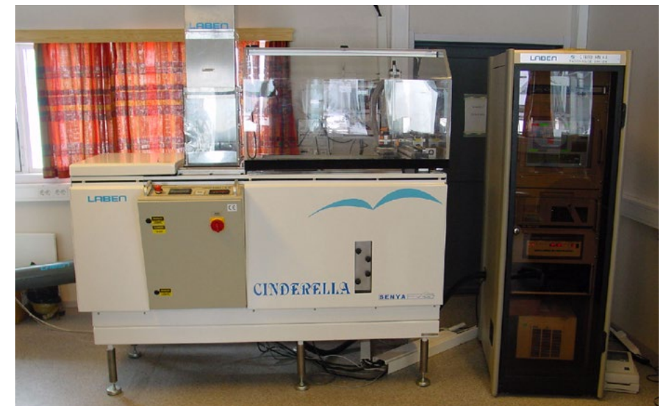
Fig 9.3.2 The picture shows the particulate component of the IMS radionuclide station in Longyearbyen, with its air sampler and detector. Paper filters are exposed for 24 hours, then rested for 24 hours, and then measured for the content of radioactive isotopes.
