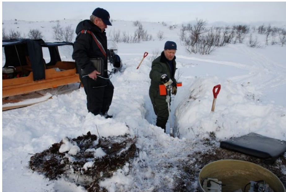
Fig 9.2.2 Preparing for the refurbishment of instrumentation at one of the seismometer sites by uncovering the vault.
