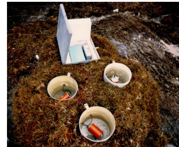
Fig. 6.3.2 This photo from the installation phase in 1987 shows one of the ARCESS three-component sites, with electronics and seismometers that record the ground motion in the vertical, north-south, and east-west directions. The picture is taken before these units are carefully covered with turf and peat moss to make the site as inconspicuous as possible.
