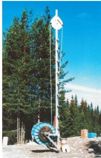
Fig 5.1.5 The three-component broadband center seismometer of the NORESS array was originally placed in a 50-meter-deep borehole.
