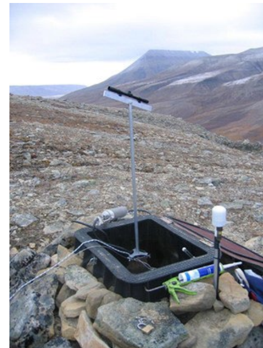
Fig. 10.2.4 The photo shows one of the instrument vaults of SPITS. The seismometer is placed in a borehole at a depth of 6 m. The photo is taken during work to align the horizontal components of the three-component seismometer in the north-south and east-west directions.
