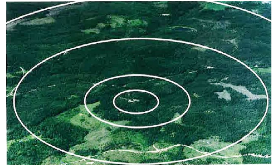
Fig 5.1.2 Aerial photo of NORESS, with the A-, B-, C- and some of the D-ring indicated (see Fig. 5.1.1). NORESS is located in a quiet forest area, at some distance from sources of background seismic noise.
